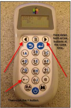
8. You will now see the channel screen. The channel that the clicker is transmitting on will appear in the upper left-hand corner. If it matches the receiver's channel that appeared in the Device Manager, then you can press enter to confirm. If the channel is different, then enter the receiver's channel # and press enter.
