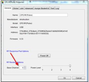
7. The clicker channel must match the base channel of the clicker receiver. To identify the channel that a clicker is transmitting on, and to change it if necessary, first turn the clicker on. Then, press the two arrow buttons at the same time. Next, press the "+" button.
